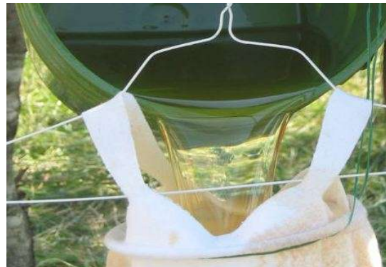
Figure 4. Filtering of waste vegetable oil for fuel.
