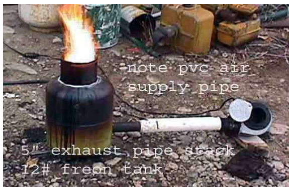
Figure 6. Example of a forced air oil burner.
