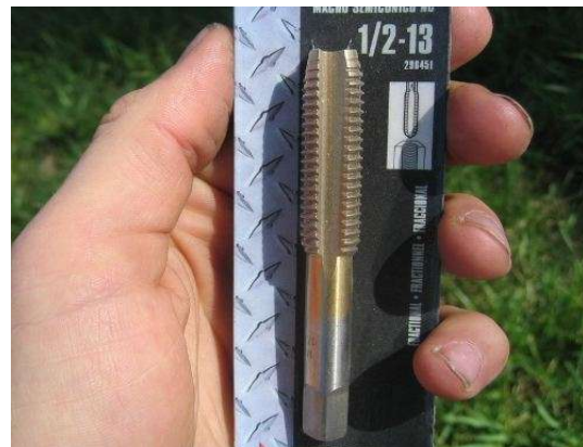
Figure 37. ½ inch tap used for making structural bolt holes.
