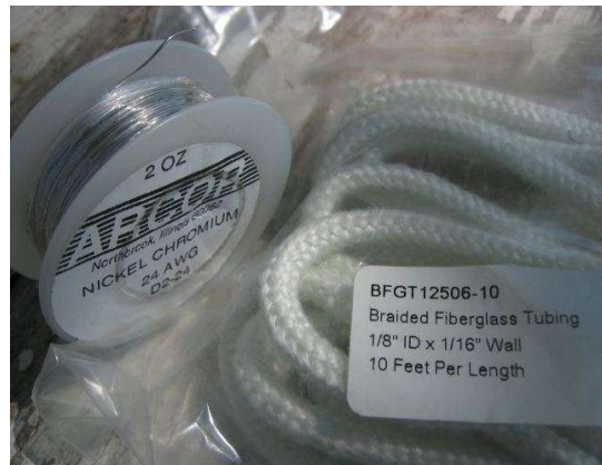
Figure 21. Nichrome wire and insulator to be used in on-demand fluid heating applications.
