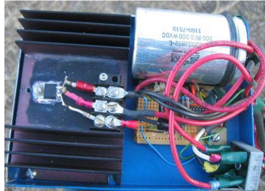
Figure 11. PWM speed controller for a 1 kW electric motor. A power-switching transistor is mounted on the heat sink.
