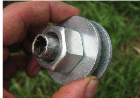
Figure 25. Modified bolt to serve as a settling tank outlet.
