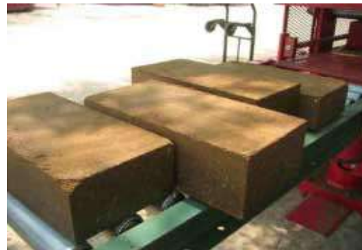
Figure 30. Finished compressed earth blocks deposited on a conveyor. 14
