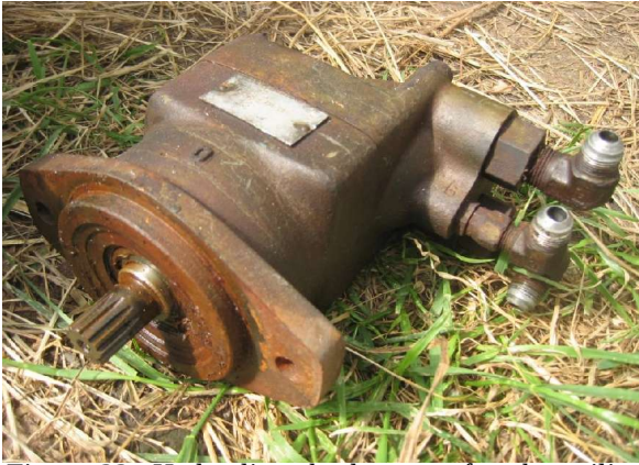
Figure 33. Hydraulic wheel motor for the utility tractor.
