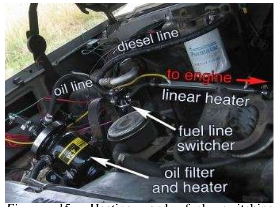
Figure 15. Heating and fuel switching components of the vegetable oil conversion.
