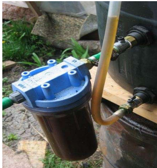
Figure 11. Basic oil filtering setup, showing the settling tank with two outlets, filter, and visor tube for checking oil quality.
