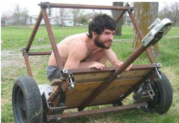
Figure 17. Power trailer frame for the VW Beetle hybrid electric vehicle conversion.
