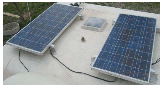
Figure 7. We use two 85 watt panels for lights and computers.
