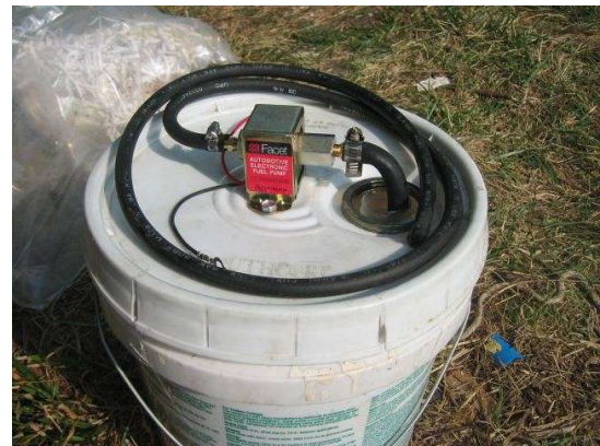
Figure 14. Priming pump mounted on the vegetable oil tank.
