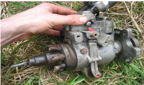
Figure 13. Original 6.2L diesel injection pump.
