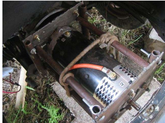
Figure 18. Advanced DC L91-4003 motor mounted on the VW Bug.
