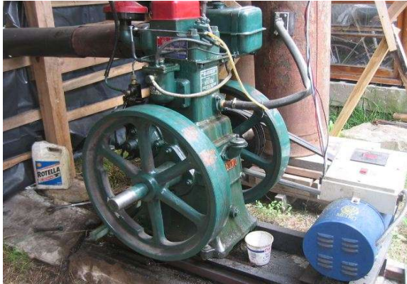
Figure 8. The Lister 6 hp, 1 cylinder diesel engine, with waste vegetable oil delivery system.
